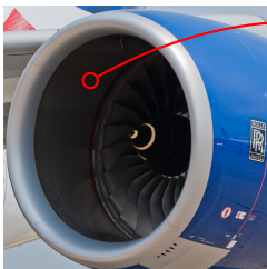
Fig. Trent 900 (A380). Inlet lined with a sound absorbing material.
