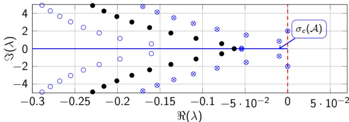
Pure delay  $g = 0$  ( $\bullet$ )  $\sigma(\mathcal{A}) = \sigma_p(\mathcal{A})$  (discrete)
